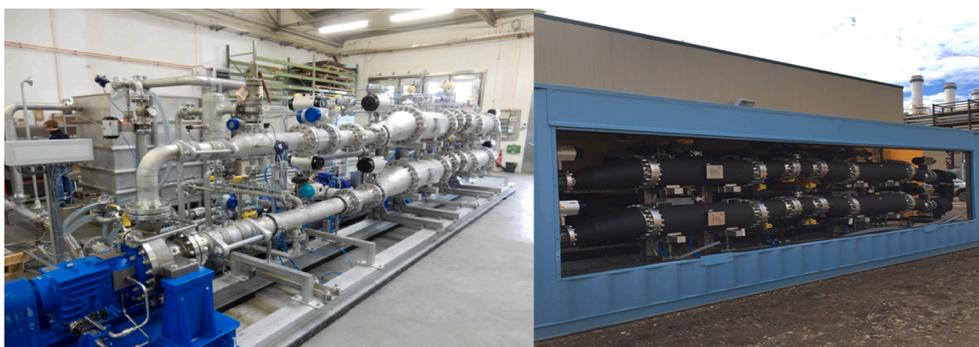
Fig. 3. Titania Nanofiltration Unit (TNU).
